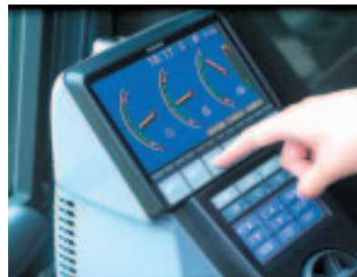
7-inch large-scale multi-color liquid crystal display
